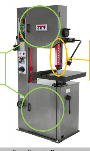
Adjustable blade guard to keep entire blade guarded except at the point of operation. This should always be adjusted to its lowest possible point.
