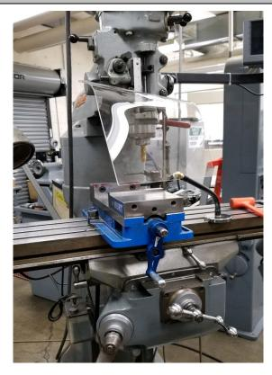
• A guard or shield that encloses the cutter head or milling bed should be utilized to protect the operator from the cutting area, flying metal shavings, and lubricating or cooling
